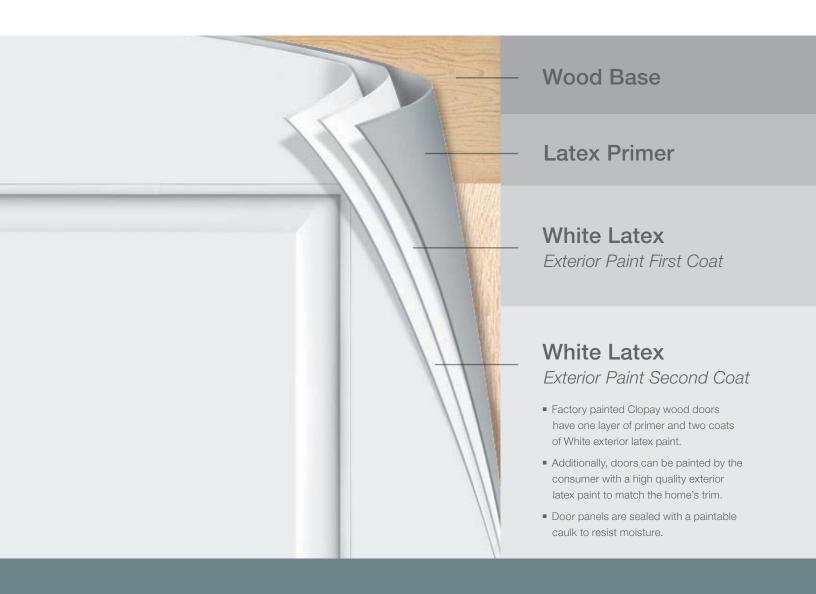
With Clopay's factory finish White paint option, your wood door arrives primed, painted and ready to install. We've eliminated the extra expense of hiring a contractor to finish the door on-site and the added worry that the job will be done right. You have peace of mind knowing that the door is stored and finished according to Clopay warranty guidelines for a durable, flawless, vibrant finish that is worthy of the most discriminating close-ups.
